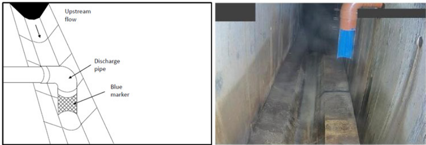
Figure 2. Example of Blue-Marker painted on cut-opened discharge pipe.
