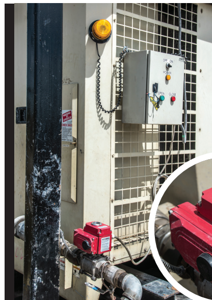
Automatic remote-control valve in operation on high pressure air compressor
